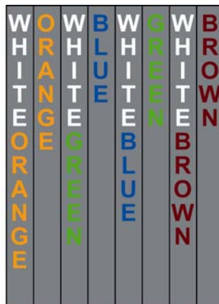
Figure 10-20 Wire arrangement of the first end of cross-over cable
