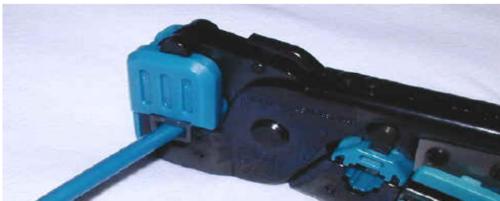
Figure 10-15 Prepare RJ-45 connector with a crimping tool
